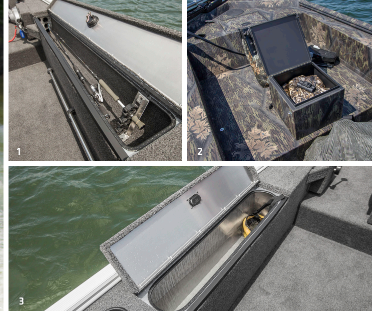
1 Starboard Locking Rod Storage 2 Tempress Seat With Storage Box 3 11-Gallon Port Side Livewell
