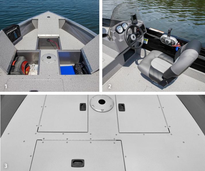
1 Bow Storage 2 Side Console Configuration 3 Optional Composite Flooring
